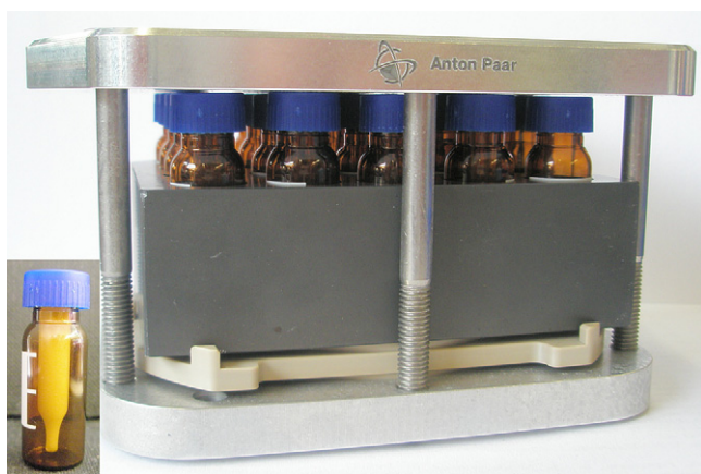
Fig. 3. Reaction platform made out of sintered silicon carbide (grey reaction block). The SiC heating platform is capable of holding up to 20 standard 200 µL screw-capped HPLC/GC vials (see insert) [17,18]. By using the corresponding rotor inside a multimode microwave reactor, four heating platforms (80 reaction vessels) can be heated simultaneously (Fig. S1 in the Supporting Information).
